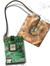
(the copper pad above) which could be installed e.g. inside the cab of the locomotive and operated by touching the outside of the locomotive.
