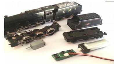
The 0554 with temporary LCU to motor lead and the experimental battery with the tender body into which they will be inserted. The 5V motor is alongside the chassis
