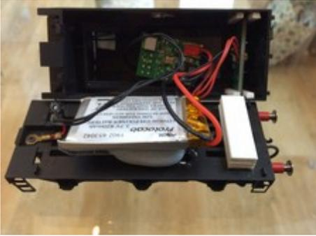
Attached photographs show installation of components in Hornby WC. tender. It all needs tidying up but works well. The battery is supported at a slight angle by blue tack. The 9601 Plug Charging Unit is a slide fit between strips of plasticard 2mm x 3mm fitted to the tender sides. It sits on a block 26mm
