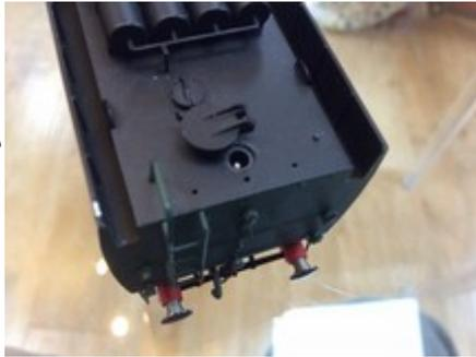
long x 8mm wide x 7mm deep. The top two outer "lands" of the board were removed to allow it to fit flush with the inside of the tender so that the socket fits in a 4mm hole drilled where the water filler cap was. This was carefully removed and then made to pivot on a 0.45mm dia. piece of wire. The 0502 LCU is fitted to the inside of the tender top under the location of the vacuum reservoir cylinders. A 9959 Heat Absorbing Pad
